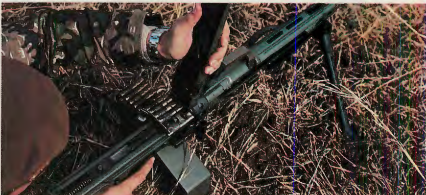
Ammunition is placed in feed tray with the open side of links outward.
